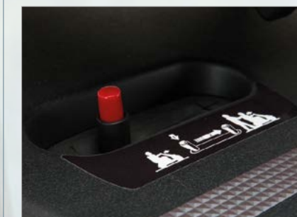
Two-step disengaging lever to prevent free-wheeling
