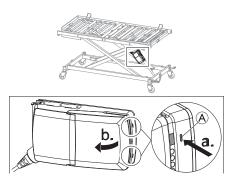
Press in the two latches (a) on the control unit with a pointed object (e.g. screwdriver) and open the lid.
